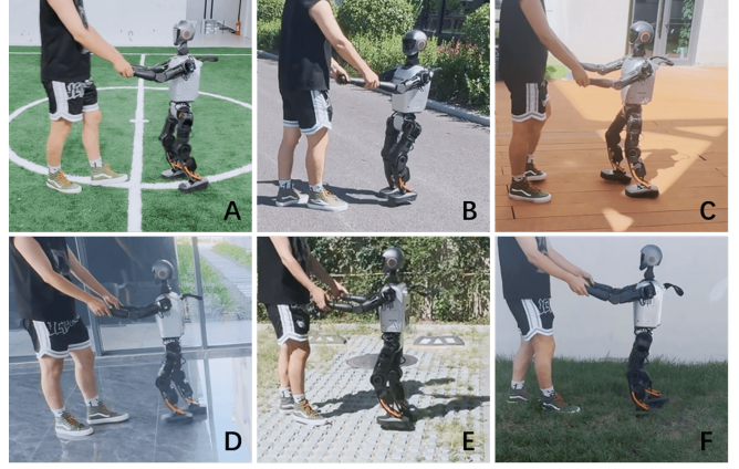
Fig. 8: Force-compliance walking in outdoor scenarios: (a) soccer field, (b) rough ground, (c) wooden ground, (d) smooth surface, (e) raised ground, (f) soft grass. The robot is guided by the human operator pulling its arms. The shoulder joint are kept flexible with a small pre-set k_p = 1 . No supportive force is exerted to the robot.
