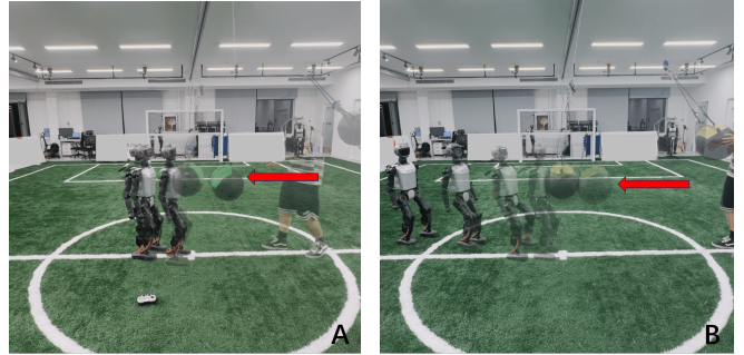
Fig. 9: Perturbation resistance under suspended-ball impacts. The red arrow represents the direction of the strike. (a) Impact of a 2-kg ball, the robot maintains balance while maintaining position. (b) Impact of a 4-kg ball, the robot steps back but remains stable.
